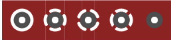
Pins with no connection, three types of thermals, and no thermal.
