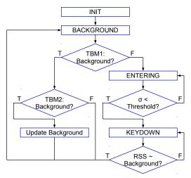
Figure 11: Flow chart for dynamic background removal.
