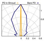
Figure 6: Vertical angular response of bare PD and PD in shroud.
