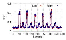
Figure 15: Time domain trace of RSS while alternately clicking a close-by and far-away point (relative to Okuli's front LED).
