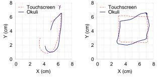
Figure 28: Okuli's virtual trackpad traces (solid) in comparison to touchscreen traces (dashed).
