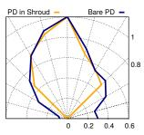
Figure 5: Horizontal angular response of bare PD and PD in shroud.
