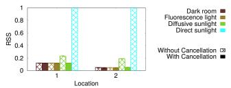
Figure 22: RSS under different lighting condition with and without ambient cancellation.
