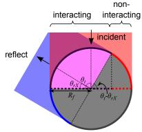
Figure 8: Modeling the *reflection coefficient* of the finger.  $R_f$  is the approximate radius of the finger.
