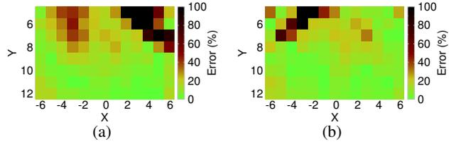
**Figure 19: Modeling error within the workspace for (a) left PD and (b) right PD. X coordinate is parallel to the LED-PD line (Okuli’s front face) and center-aligned with the LED. Y coordinate denotes the distance from the LED-PD line.**
