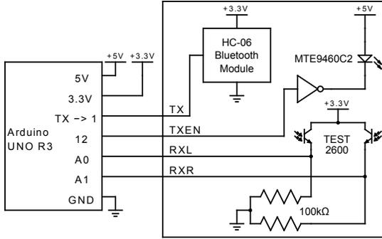
**Figure 18: Simplified schematic of the Okuli experimental prototype.**
