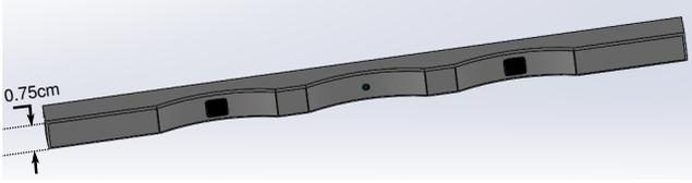
**Figure 3: Concept-art of a product version of Okuli, to be fit into the edge of a small mobile device with a thickness around 7.5mm.**
